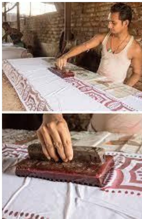
Figure 3: Waxing the area of the fabric
