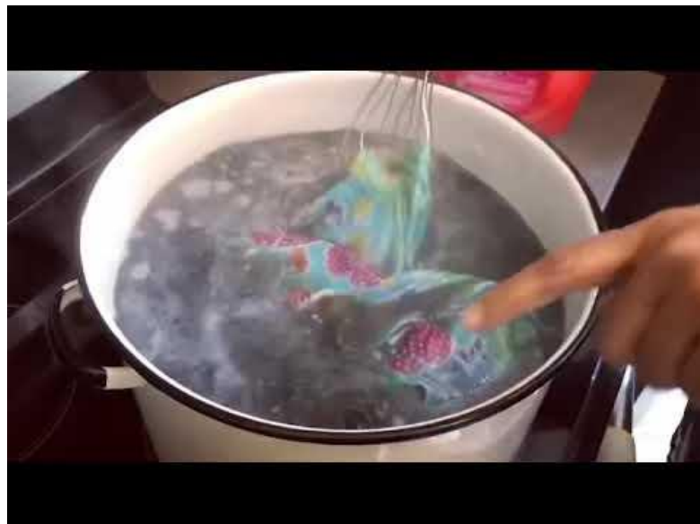
Figure 5: Removing the wax from the fabric
