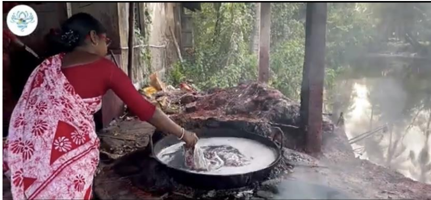
Figure 6: Washing the fabric to remove residual soap
