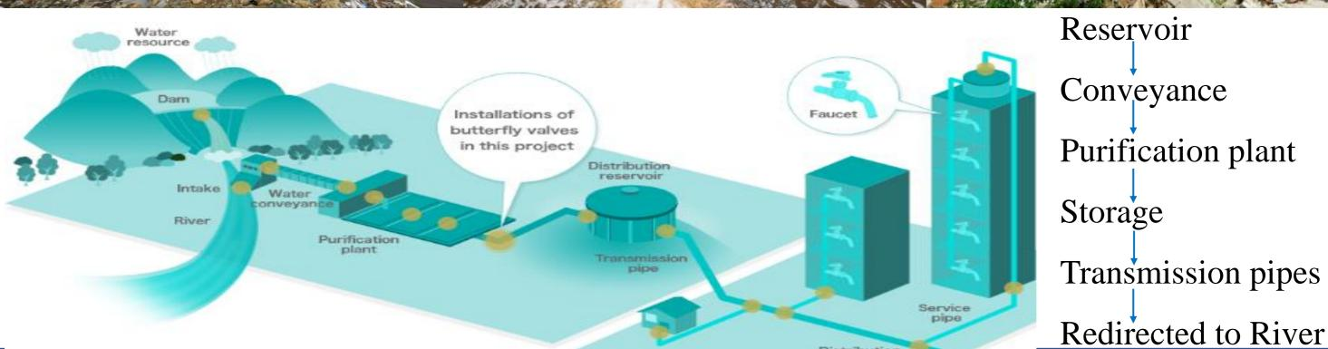
Reservoir Conveyance Purification plant Storage Transmission pipes
