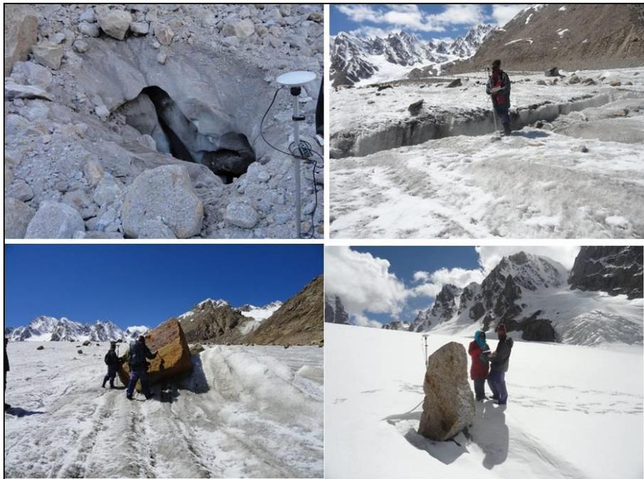
Figure 260: DGPS measurements over the ablation zone of the Chhota Shigri glacier in Himachal Pradesh
