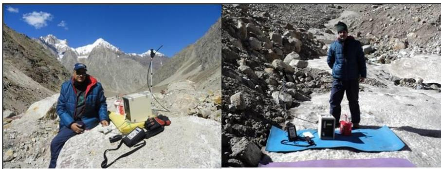
Figure 261: Aethalometer measurements over the ablation zone of the Chhota Shigri glacier in Himachal Pradesh
