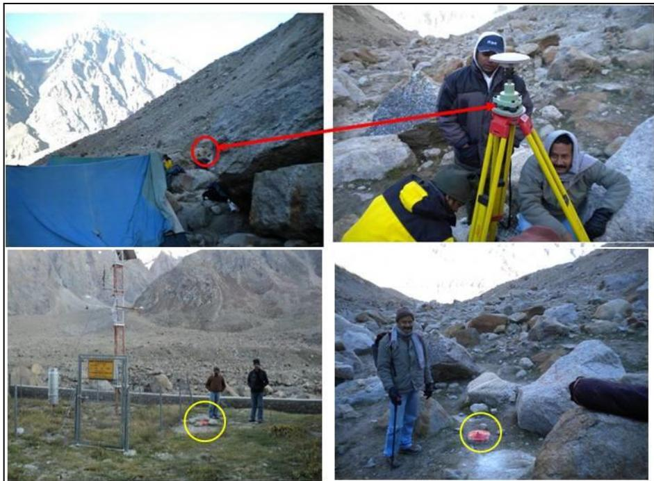
Figure 263: Establishment of DGPS Base stations and rover near the snout of Chhota Shigri glacier in Himachal Pradesh
