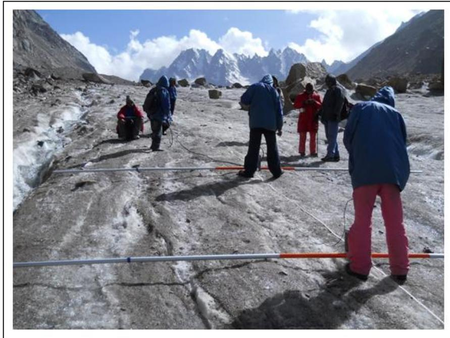
Figure 221: Operation of MLF antenna on ablation zone of Chhota Shigri glacier (Source: Singh et al., 2012)
