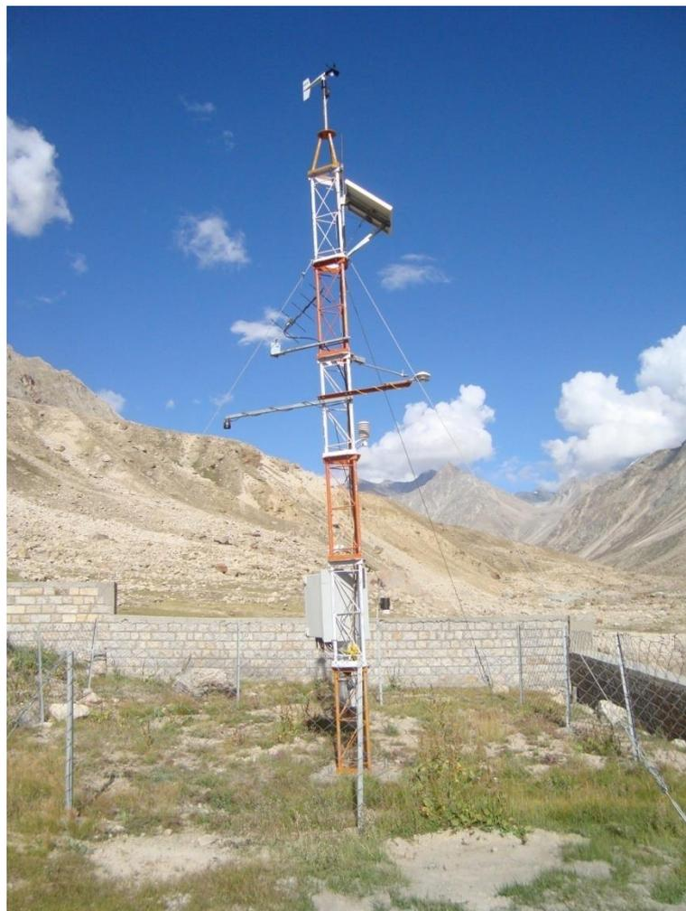
Figure 270: AWS installed at Chhota Darra near Chhota Shigri glacier, H.P.
