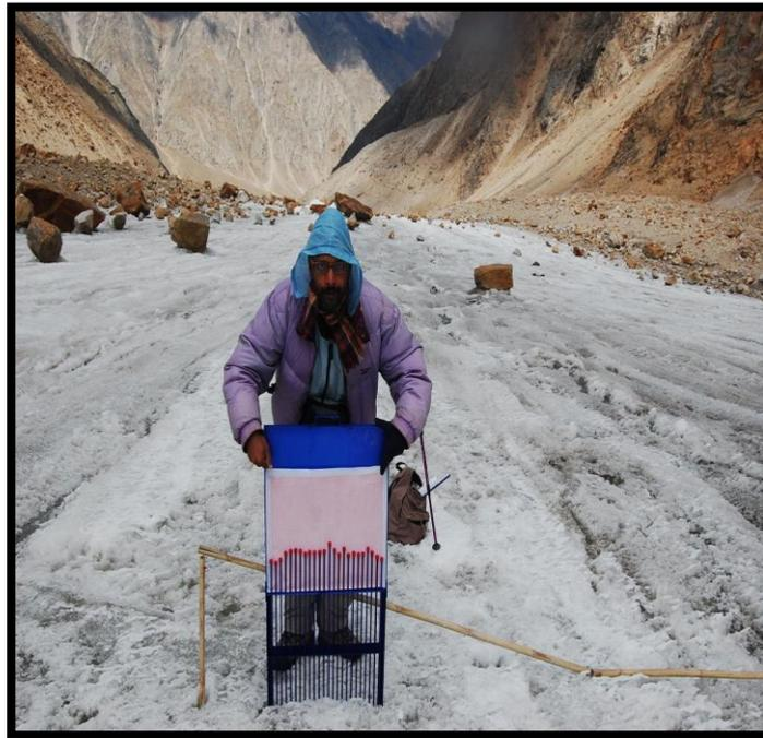
Figure 313: Measurement of roughness on glacier with profilometer
