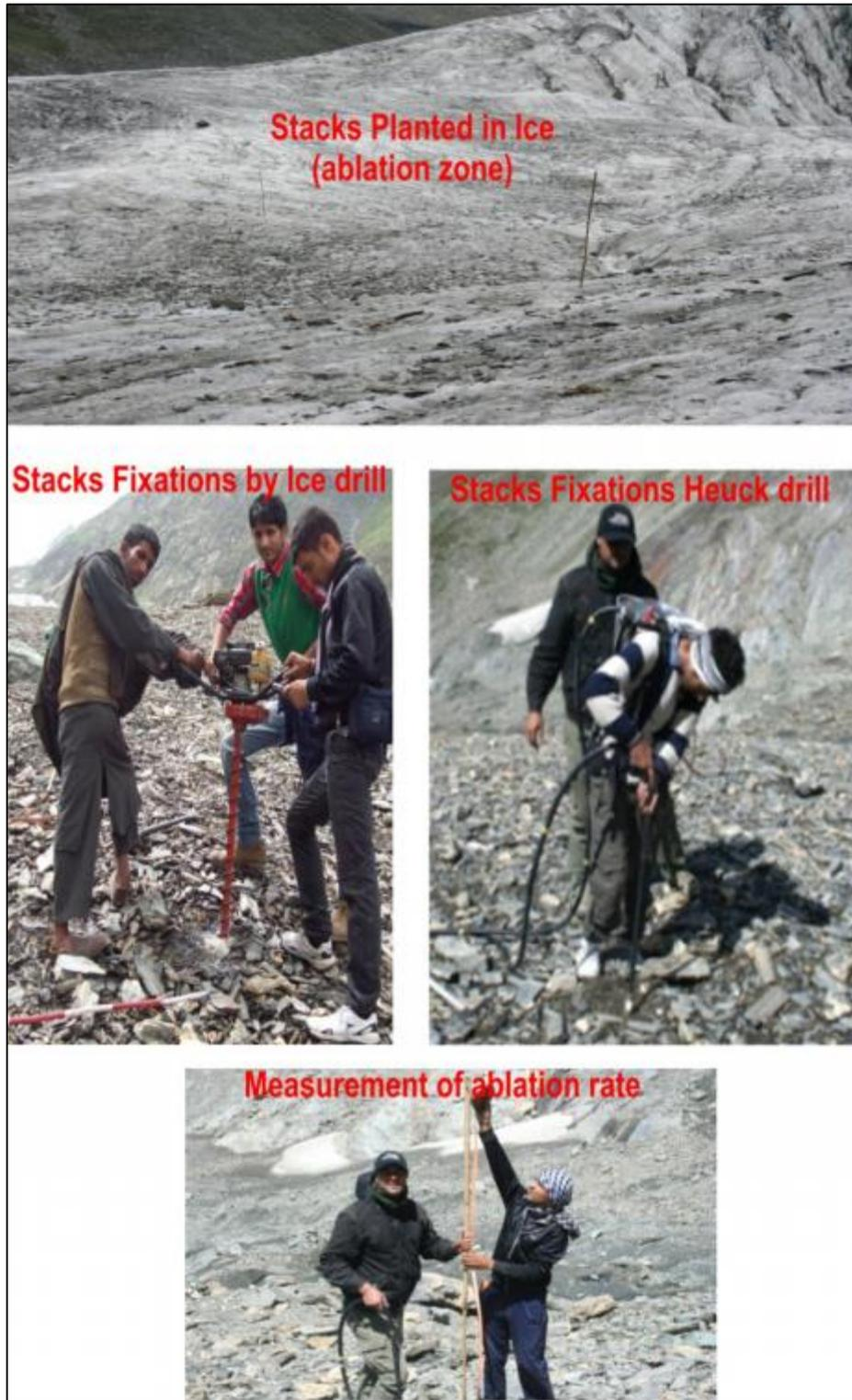
Figure 185: Fixing of ablation stacks and measurements on Machoi glacier
