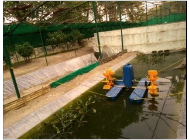
Experiment with paddle aerators
