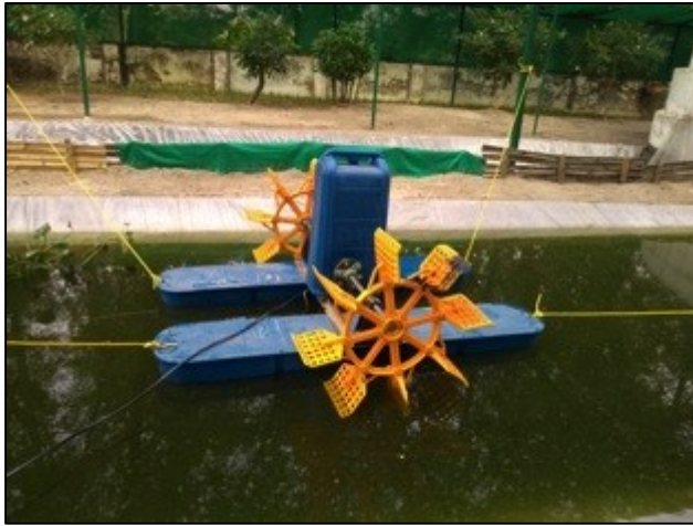
Experiment with paddle aerators
