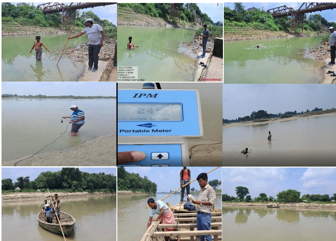
Figure B.6 Measurement of suspended sediment concentration and river cross-sections
