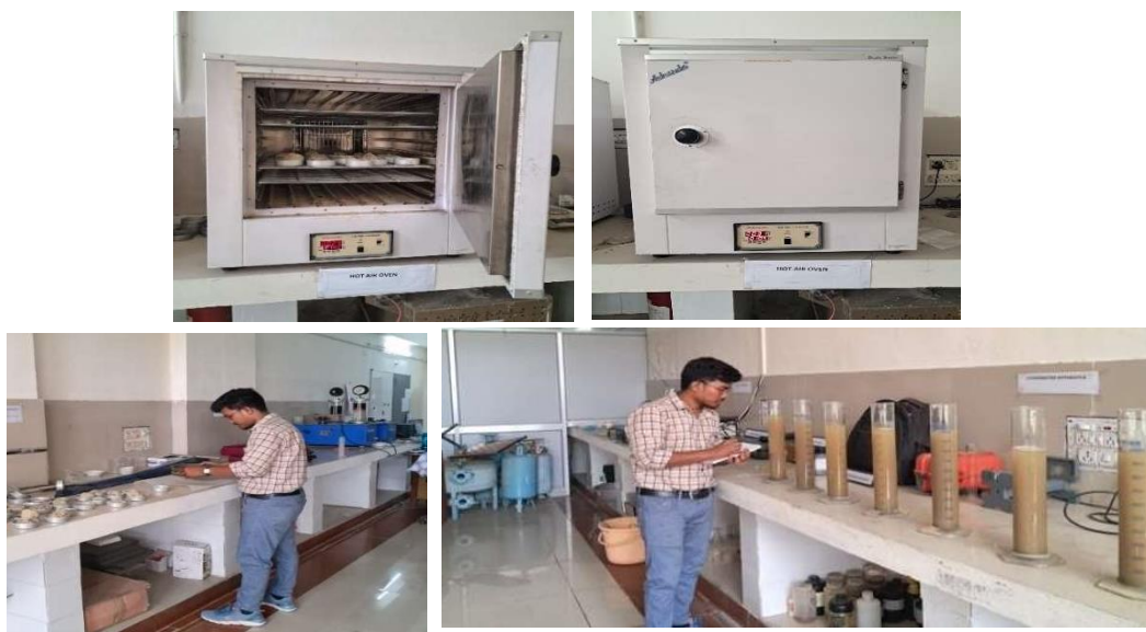
Figure B.4 Hydrometer Testing of soil sample
