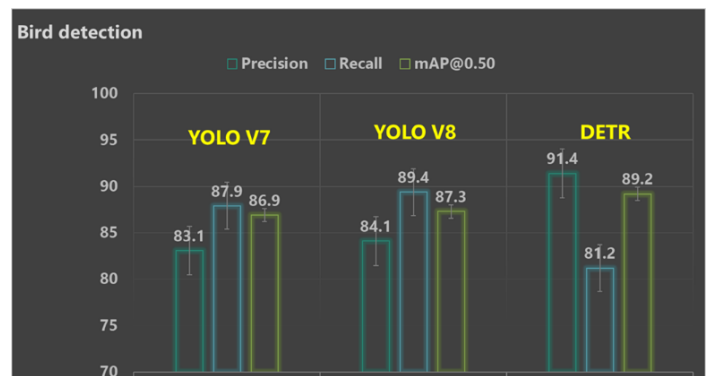
Fig. 5. The precision, recall, and mean average precision graphs illustrating bird detection are presented for three models. DETR successfully detected birds, as indicated by its accuracy.
