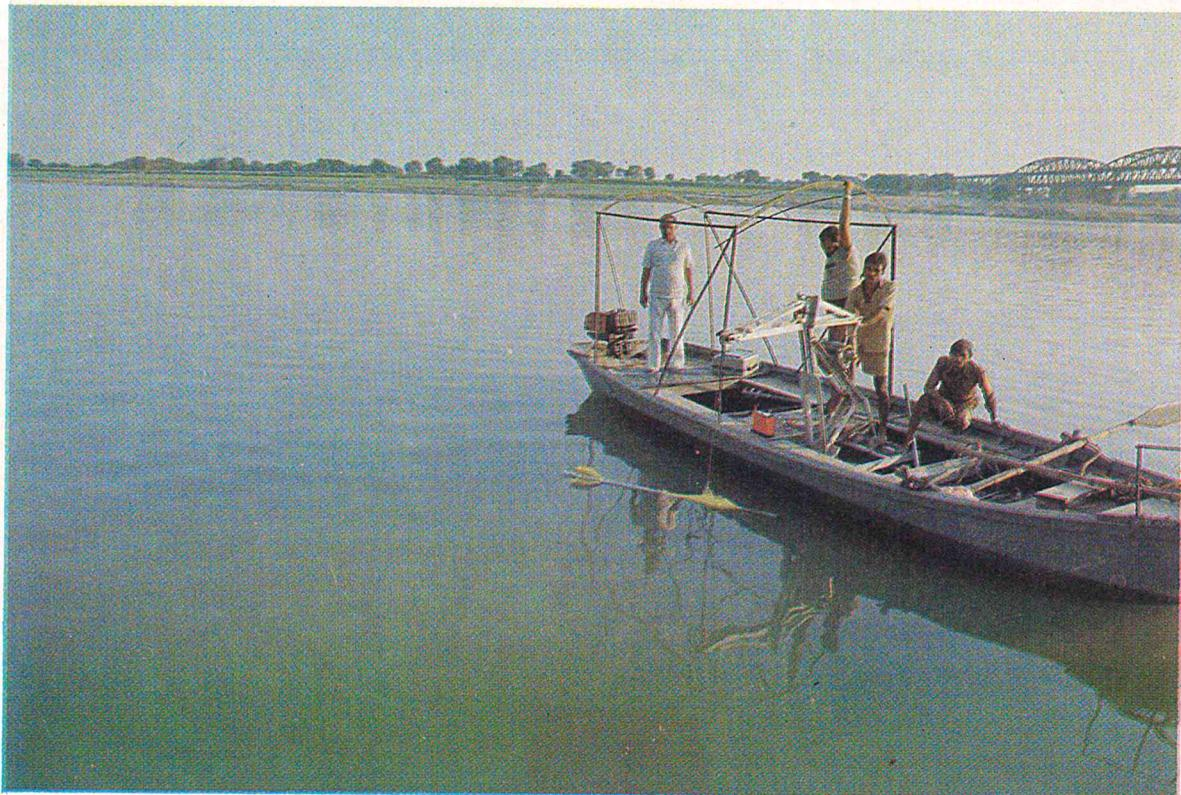
Velocity Observation using A. OTT Propeller Type Current Meter
