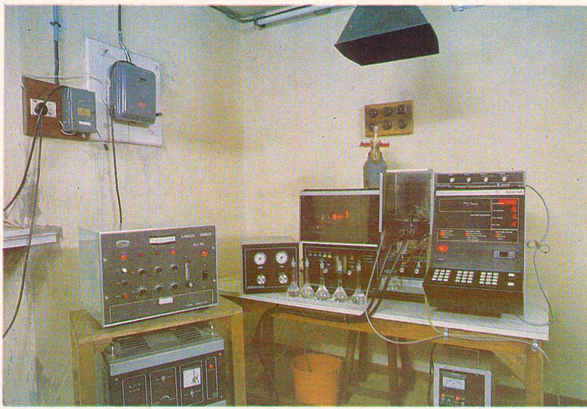
Model 850 Double Beam Atomic Absorption Spectro-photometer
