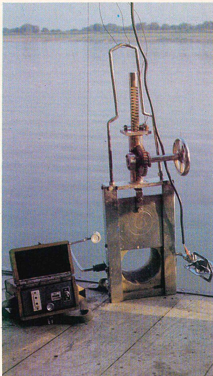
Plankton Sampler Fitted with Pigmy Current Meter
