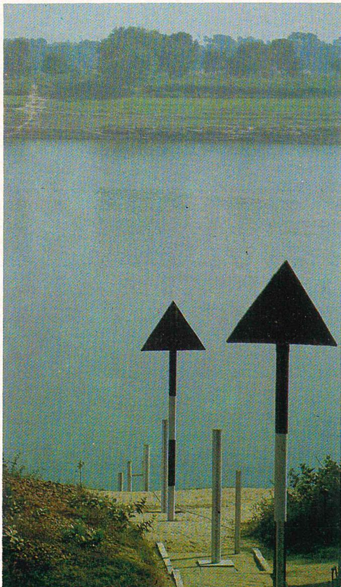
Wooden staff Gauges and Targets Measuring Cross Section in Ganga
