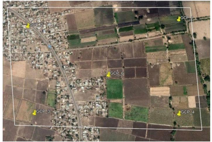
Figure: Drone AOI with GCP placement
