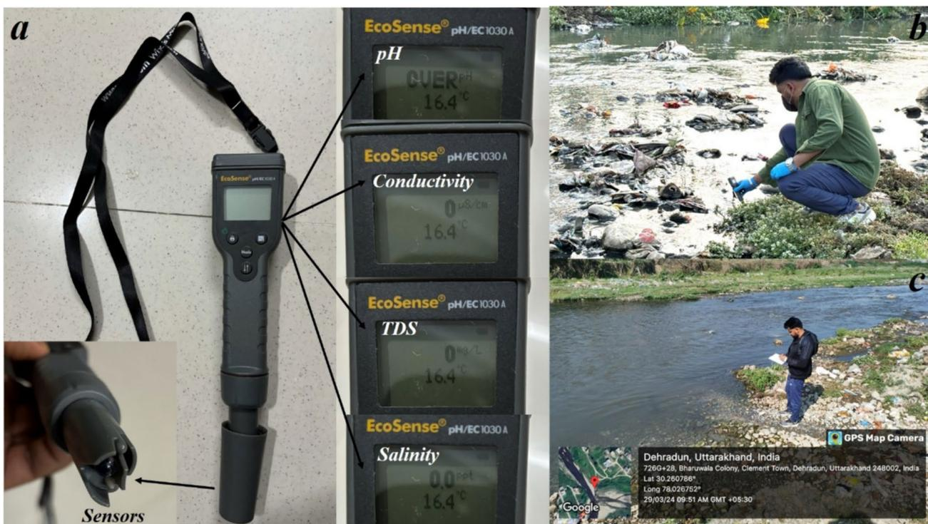
Fig. 2 a Photograph of YSI EcoSense pH/EC 1030 A instrument. b, c Photographs taken during the field survey
