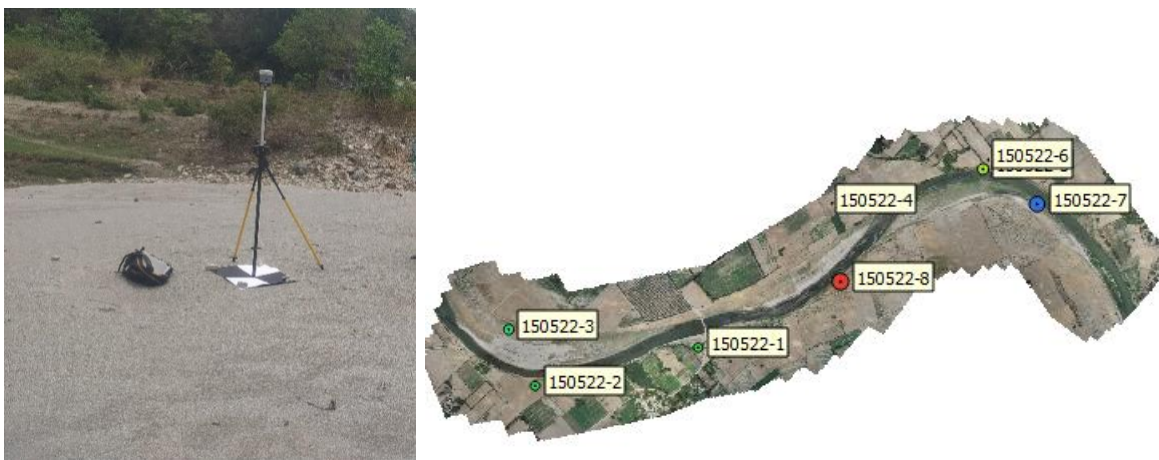
Figure 3. Left figure shows the marker used as GCPs in the river floodplain and the figure on the right shows the distribution of GCPs in a site.
