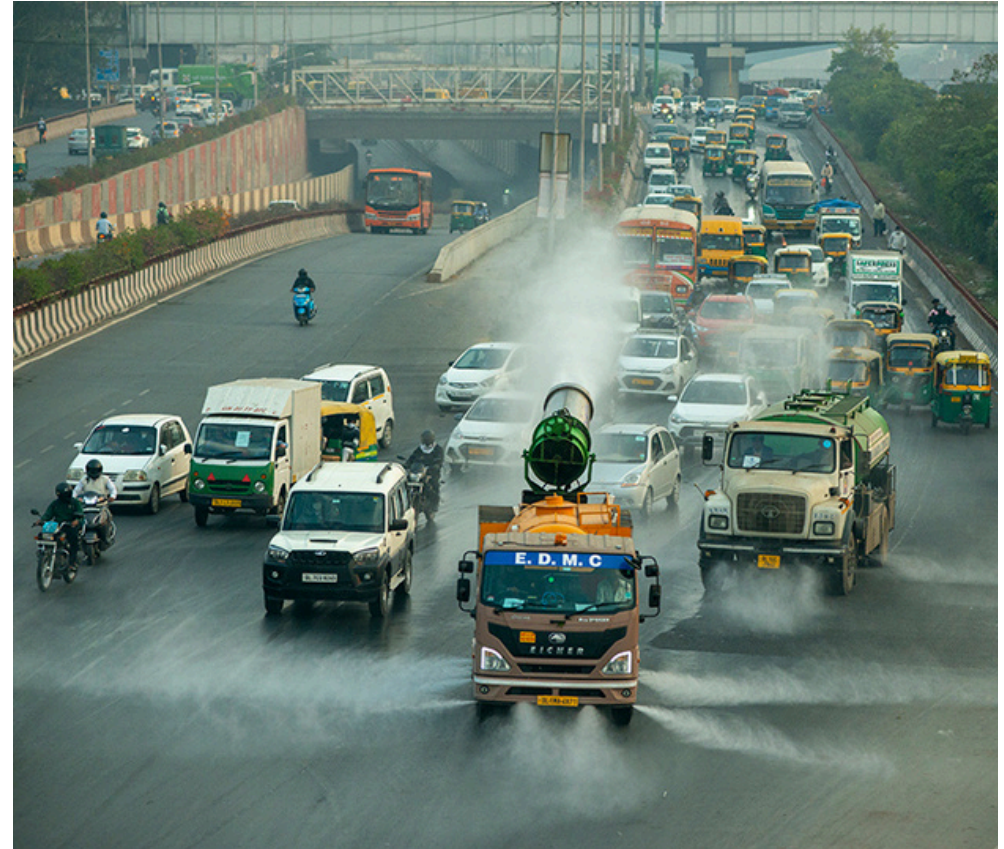
Anti-smog gun used for dust suppression. Chief Minister on the issue of air pollution Source: Pradeep Gaur/SOPA Images (2020)
