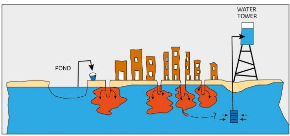
Figure 14-6: Domestic water and groundwater in a rural village. Groundwater is also recharged by waste water.
