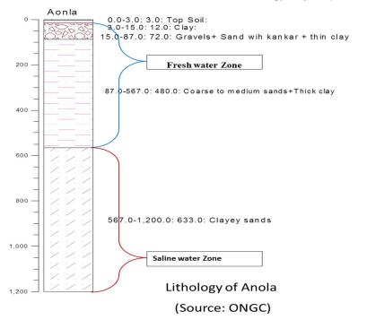
Figure 15-5: Fresh – saline groundwater interface in deep ONGC boreholes (ONGC/CGWB).
