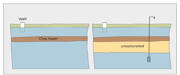
Figure 17-15: Examples of "normal" (left) and "perched" (right) groundwater situation (blue = groundwater)
