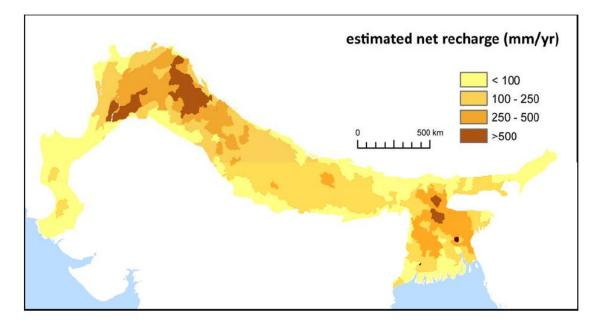
Figure 17-7: Net recharge, calculated by subtracting the calculated annual water storage change from abstraction. Net recharge will be equivalent to the groundwater recharge minus natural discharge to rivers (Bonsor et al., 2017).
