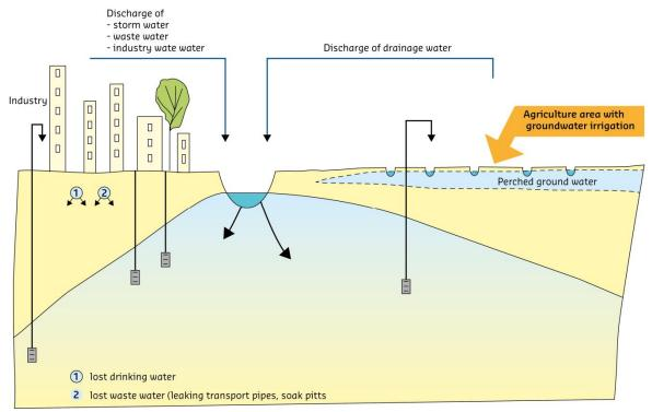
Figure 18-1: Different groundwater surface water interaction possibilities.
