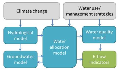
Figure 8-1: Flow diagram with the components of the river basin model and the link to the e-flow indicators, scenarios and strategies
