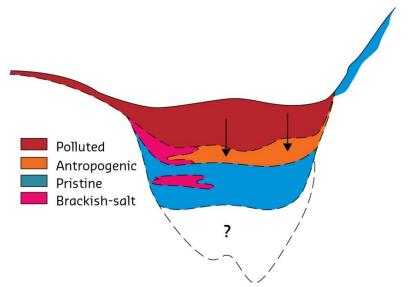
Figure 0-11: Schematic presentation of vertical zoning of general water quality types. Below the pristine water zone. Saline water is observed in some deep oil borings.
