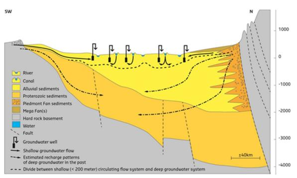
Figure 14-11: Conceptual geology and groundwater flow conditions in Ganga basin.
