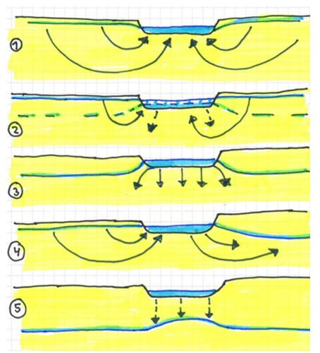
Figure 18-2: Different possible river – subsurface flow interactions.
